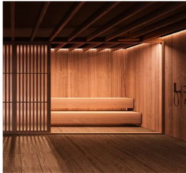
LED INSTALLED UNDER SAUNA SEATS TO SOFTLY WASH DOWN AND CREAT AMBIENCE
