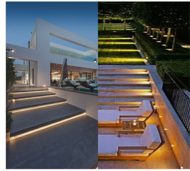
LED INSTALLED UNDER EXTERNAL STAIRS TO CREATE A FLOAT EFFECT PIN LIGHTS INSTALLED AS LOW LEVEL LIGHTS TO SOFTLY WASH ACROSS EXTERNAL PATHWAYS
