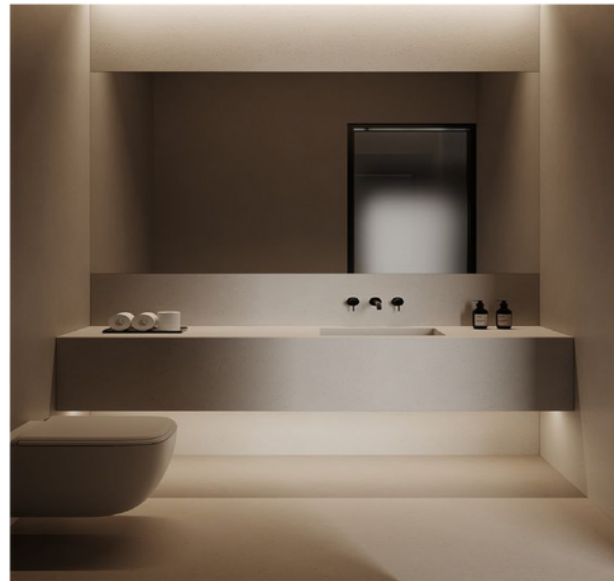
LED INSTALLED UNDER BATHROOM VANITIES TO CREATE A SOFT FLOAT EFFECT
