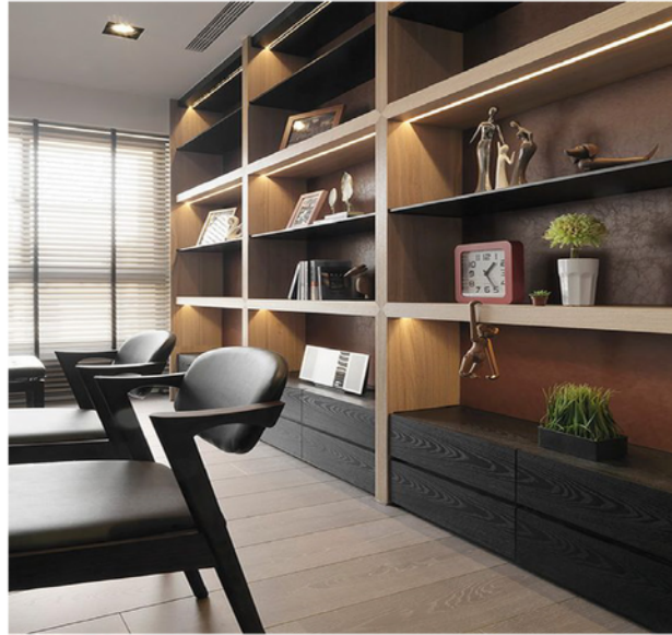
MICRO LED INSTALLED IN OFFICE JOINERIES TO HIGHLIGHT BOOKS AND FEATURES
