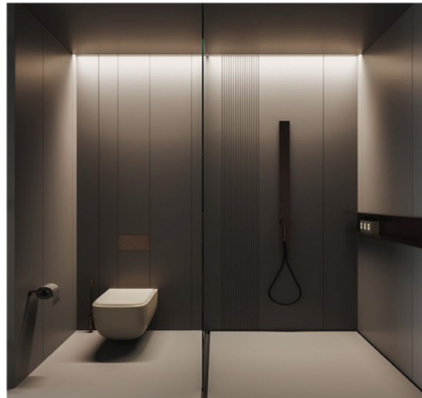
LED INSTALLED IN SHOWER CEILINGS TO SOFTLY WASH ONTO WALLS
