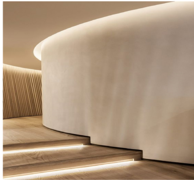
FLEXIBLE LED TO WASH FEATURE CURVED WALLS IN HALLWAYS AND THROUGHOUT
